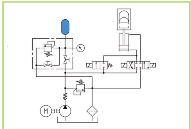
Safety devices enter into function in case of breakdowns. They shut partitions, valves, by-passes or hopper valves, silos or conveyors. These devices can also control stop valves of foundry aggregates or ladles, as well as open and close high capacity circuit breakers. Normally the accumulators used in these applications are inactive. They are filled with oil, buffering energy which is immediately available on demand.
