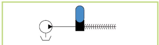
Hammering cannot always be damped at the source. It is often very difficult to find their origin, and, even worse, they propagate themselves all over the hydraulic system. Pulse-Tone accumulators help protect the pump as well as the testing devices against hammering.
