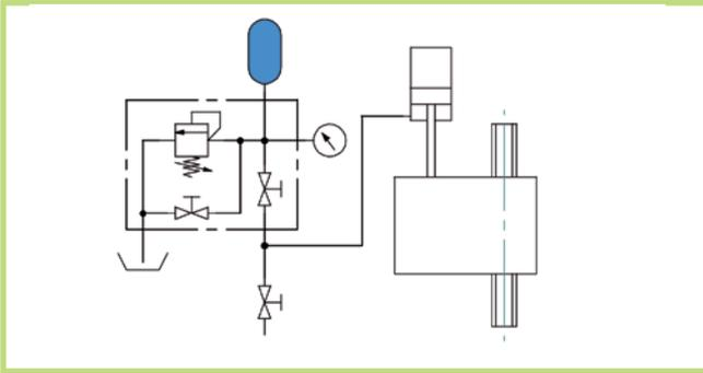
Small dimensions, inertia free accumulators can be used for balancing heads of machine-tools. Compared to a counter-weight system with chains, the hydraulic balancing using an accumulator offers the following advantages: weight reduction, lesser vibrations transmitted to the foundations, more compact solution, easier to transport, higher adaptivity thanks to the possibility of varying the gas filling pressure.
