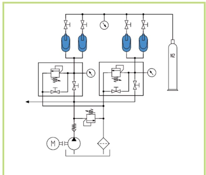
In certain installations, often only small differential pressures can be tolerated (e.g. in injection moulding machines). In other cases (e.g. in rolling mills), important quantities of oil must be accumulated. In both cases great volumes of gas are required. Cost can be reduced by using transfer accumulators connected to pressurised gas cylinders.
