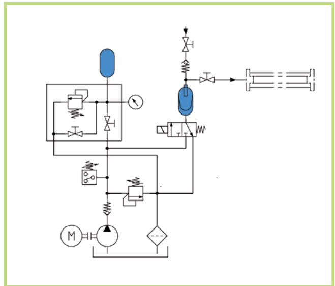
In case of leaking pipe systems, pressure tests (for instance for high-pressure pipes) are mostly used with water which is less contaminating than oil. In order not to have to build stainless-steel pumping units a standard hydraulic unit connected to a transfer accumulator is used (an additional standard accumulator is used to maintain the pressure and prevent the pump from having to run continuously).
