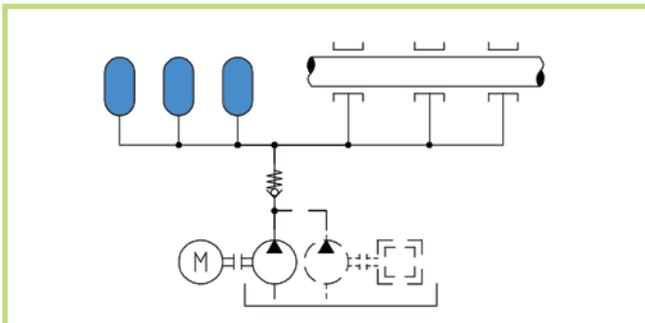
Bearings of big machines such as turbines, compressors and very high capacity water pumps must be constantly lubricated. When mains fail emergency pumps driven for instance by a diesel motor must immediately enter into operation. When starting, the auxiliary pump receives no lubricant during a few seconds. OLAER hydraulic accumulator enter at this precise moment into service and secures a constant pressure of the lubricating oil.
