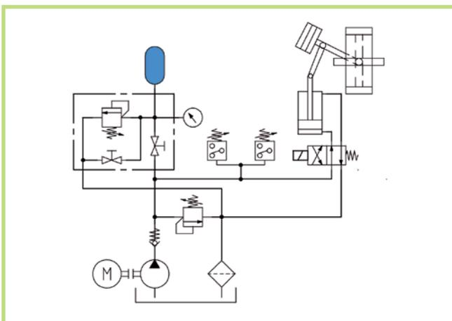
Oil leaks cannot be avoided in hydraulic systems where high pressures have to be maintained for long periods (examples: throttle valves which are maintained open by means of a spring or a counterweight, chucking systems or pressure tests). Oil topping has to be constantly secured.
