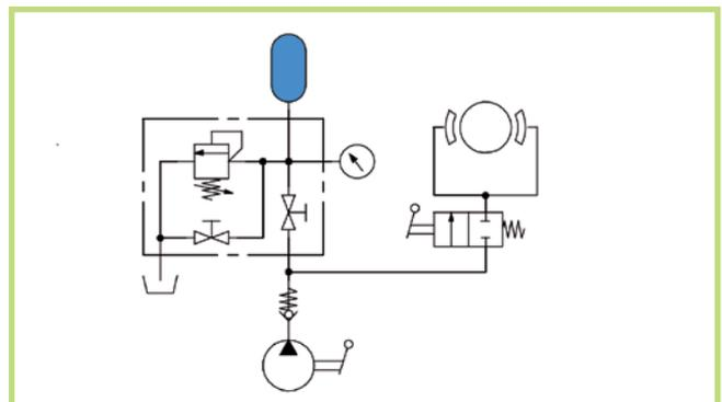
Hydraulic accumulators can for instance be used to control emergency brakes or funicular railway, gondola or bus doors. The accumulators being charged at the station by means of a motorised pump or in emergency case by a hand-pump. The necessary energy is therefor constantly available to carry out an emergency stop. Often, the command is inverted, braking being carried out by a spring, the accumulator keeping the cylinder operated braking caliper open.
