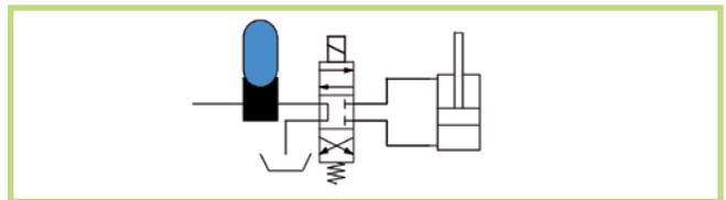
Fast running machines cannot always run "smoothly". Pulse-Tone series accumulators are used here to absorb shocks.
