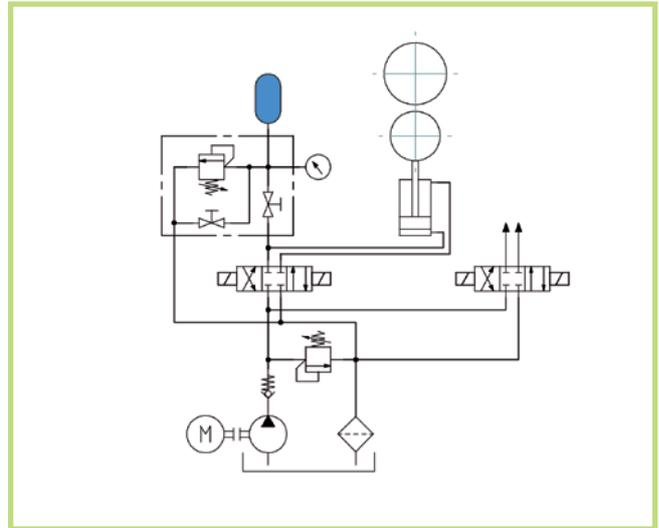
Accumulators can be used to maintain the mechanical pressure applied between two rolls. After having reached the required pressure the pump can be immediately switched to other users, the hydraulic accumulator securing the pressure between the rolls during the entire process.
