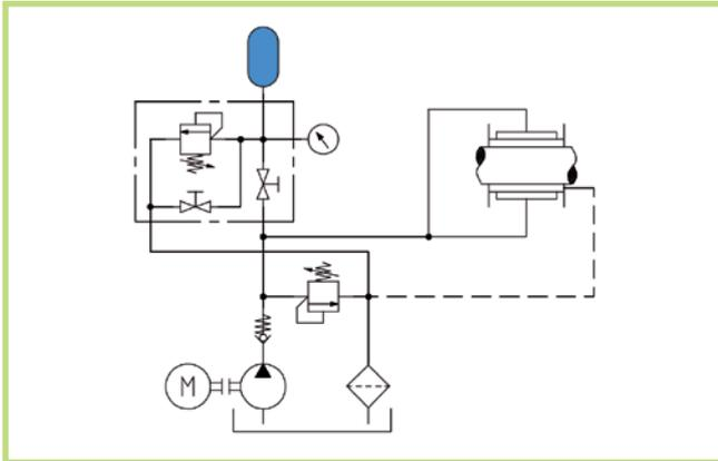
Hydrostatic bearings on machines must be held under pressure. In case of a mains breakdown the pumps stop and the oil pressure falls. OLAER hydraulic accumulators maintain a minimum pressure up to the complete halt of the machine and avoid expensive bearing damages.
