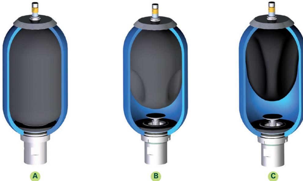
The bladder is filled with nitrogen through the gas valve and takes the shape of the accumulator shell **A**. By pumping hydraulic fluid into the accumulator, the gas contained in the bladder will be compressed. The gas volume is reduced and pressure increases. Hydraulic fluid accumulates in the unit **C**. Conversely, the accumulator will empty itself as soon as the hydraulic fluid pressure is lower than the gas pressure **B**.
