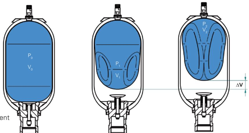
Piston and diaphragm accumulators use the same operating principles with different constructional principles.
